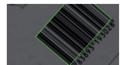
Reading strongly blurred bar codes
