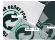
HALCON's advanced matching technology even finds objects which are partially occluded
